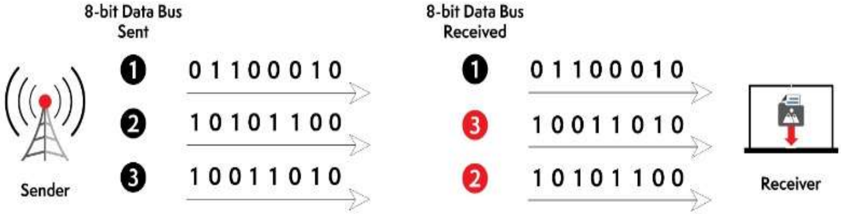
Example of Parallel Transmission - Data Received Incorrectly
